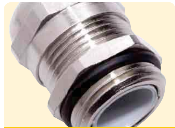
Fig. 3b: Special outdoor seal, still in good condition following ozone/UV test
