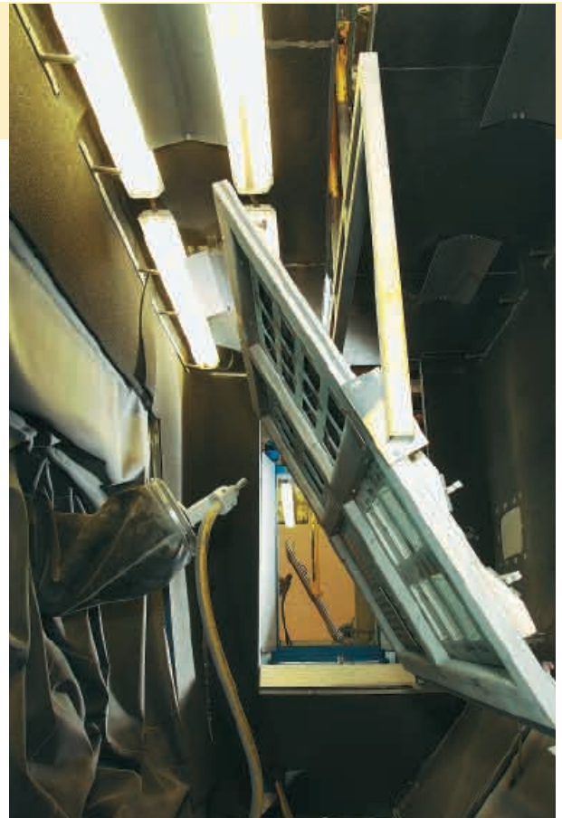
Surface activation through bombardment with granulated particles
